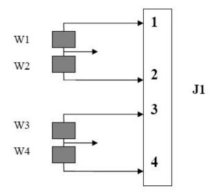
FIGURE 2.4 SIX LEAD MOTOR - FULL WINDINGS CONNECTIONS
