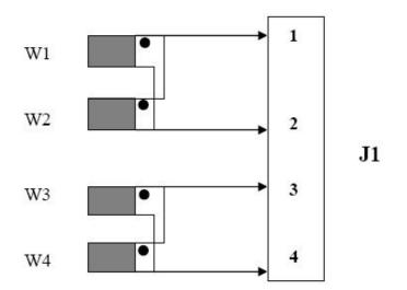
FIGURE 2.6 EIGHT LEAD MOTOR - PARALLEL CONNECTIONS
