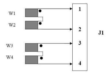
FIGURE 2.5 EIGHT LEAD MOTOR - SERIAL CONNECTIONS
