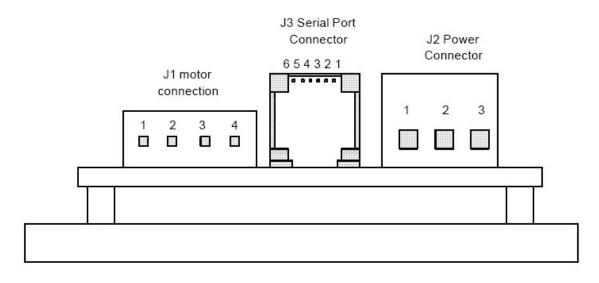
J1 Motor Connection pin 1 = winding <u>A</u> pin 2 = winding A pin 3 = winding <u>B</u> pin 4 = winding B J3 Serial Port Connections: pin 1 = not connected pin 2 = TX (data into SMC) pin 3 = RX (data out of SMC) pin 4 = must be left open pin 5 = GND (signal reference) pin 6 = not connected
