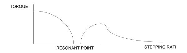
Actual ramping rate in step/sec/sec is calculated by formula:
