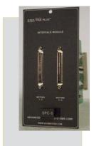
The Step Pak Plus SPC-5 Interface Module provides two front panel connectors for direct connection to the Pro-Dex MAXv-8000 indexer/controller. One-to-one connectivity from the Step Pak rack and Step Pak stepper or servo modules to the MAXv makes drive and control quick and easy.
