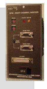
The Step-Pak SPI-8 is an 8-Channel Indexer Module that plugs into the Step-Pak System Rack and provides step and direction output for up to 8 Step-Pak Motor Driver Modules. Home, Limit+ and Limit- inputs are available for each channel. Additionally the SPI-8 supports eight status inputs and eight control outputs via front panel connectors. Communications with the host computer is via RS-232 or RS-485 communications ports.
