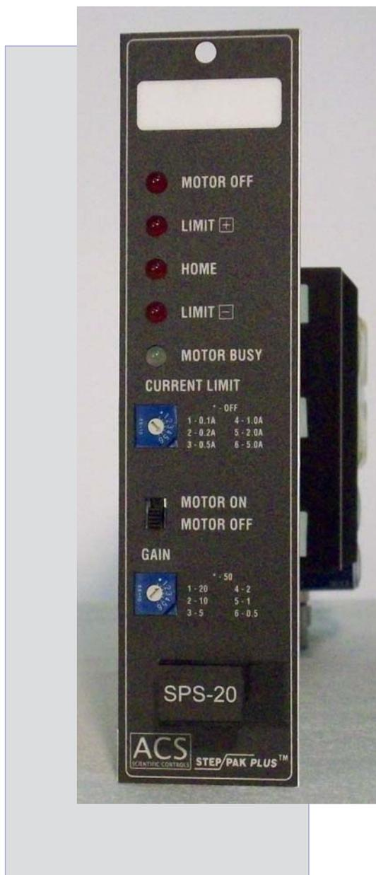
The Step Pak Plus **SPS-20** is a servo amplifier module that plugs directly into the Step Pak System Rack providing drive current for DC servo motors.
