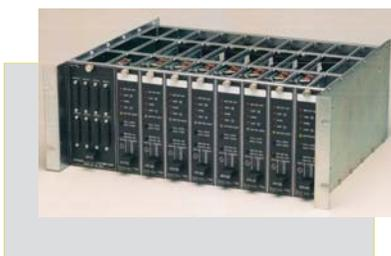
The **Step Pak Modular Motion Control System** is designed for the drive and control of up to 8 (eight) motors. Well suited for control scenarios using different sizes and types of stepping or servo motors in the same application, the **Step Pak System** provides Scientists with economy, flexibility and scalability
